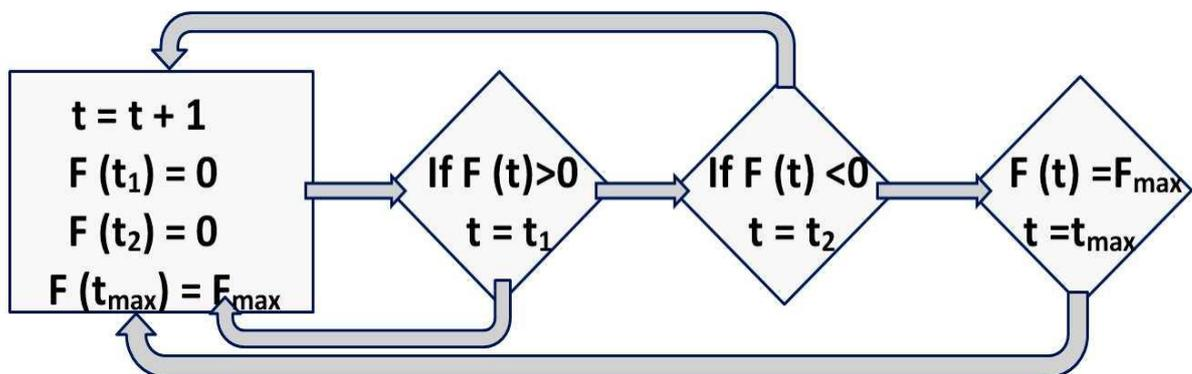
Figure 2. Block diagram of the computer algorithm for determination of  $F_{max}$ ,  $t_1$ ,  $t_2$ ,  $t_3$
