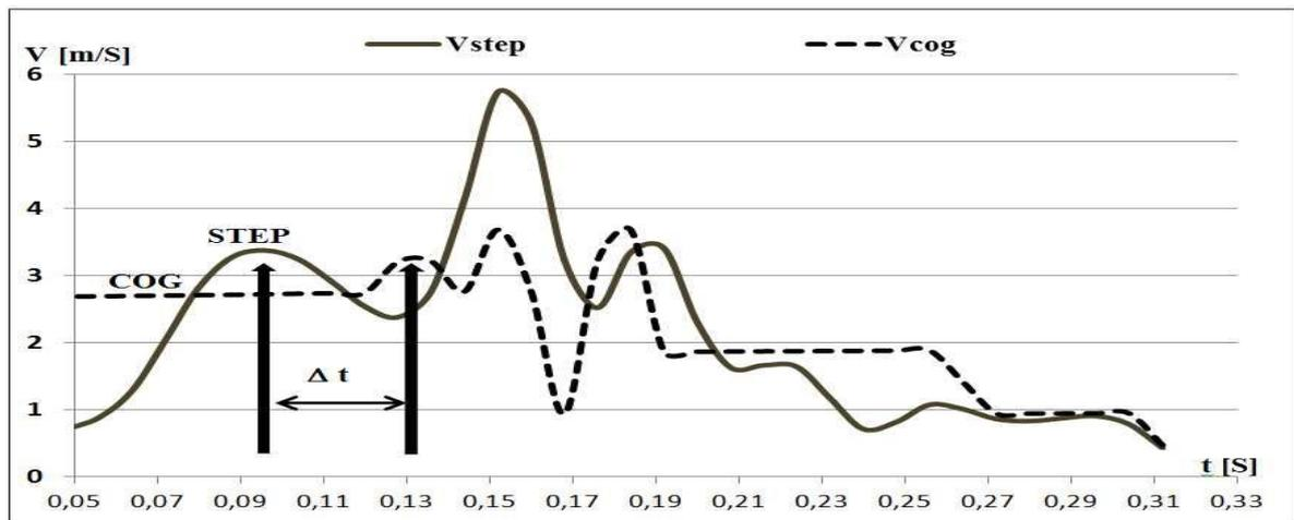
\***Vstep** - Velocity of the step in the vertical rebound of the lower limb
